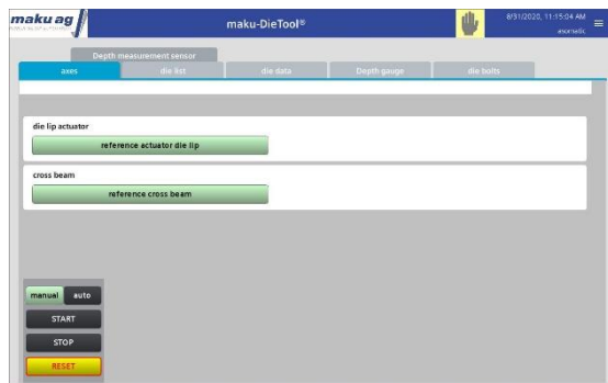
Figure 5: reference die lip actuator and cross beam
