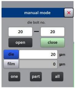
Enter the first bolt and the last bolt of the adjustment
