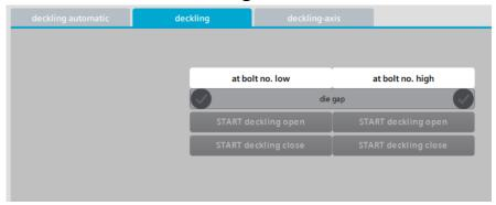
→ enter the actual value of the deckling blade in "deckling gap"
